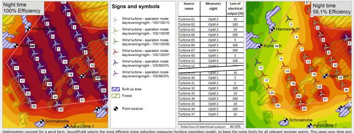
Optimization concept for a wind farm. SoundPLAN selects the most efficient noise reduction measures (turbine operation mode), to keep the noise limits for all relevant receiver points. This saves your time and assures the highest electrical output possible
