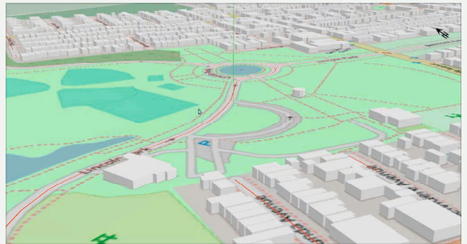
Map interface with integration of Google Maps and OpenStreetMap for easy selection of the investigation area. Enables direct transfer of background maps and/or geospatial data for accurate positioning and context.
