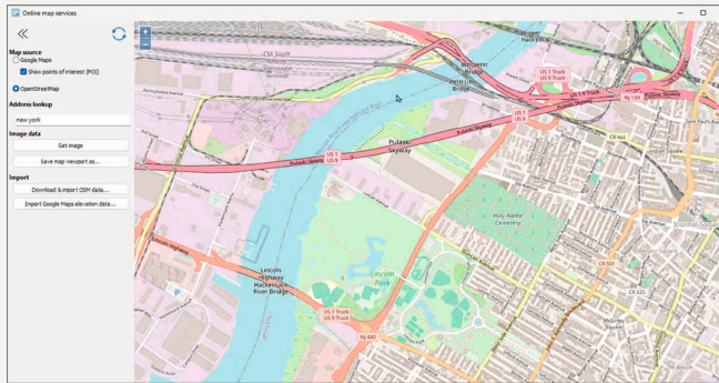
Map interface with integration of Google Maps and OpenStreetMap for easy selection of the investigation area. Enables direct transfer of background maps and/or geospatial data for accurate positioning and context.
